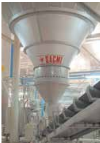
Cone with Internal anti-wear lining (optional)
