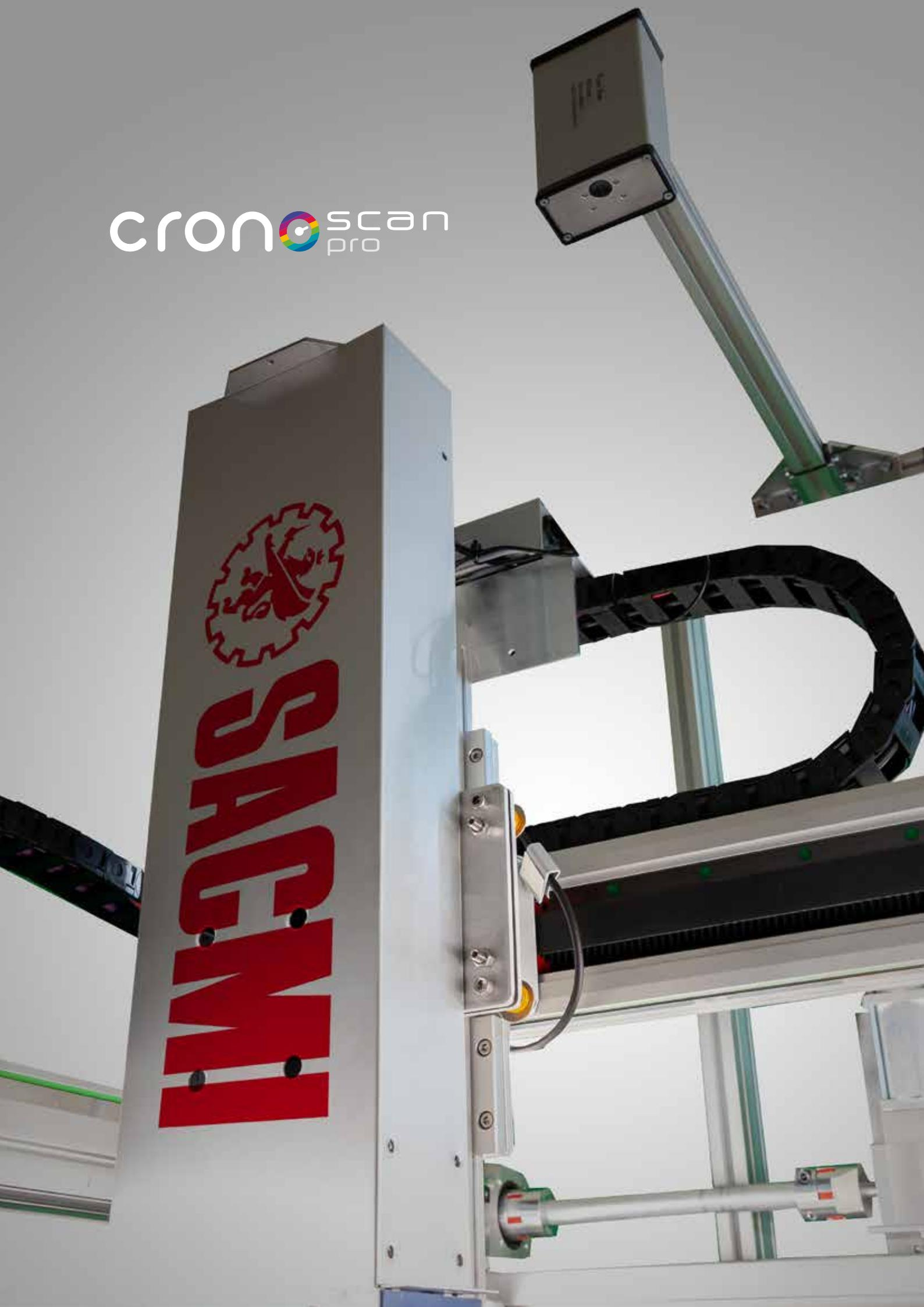
**CronoScan PRO:** next-gen spectral scanner, designed for the professional acquisition of both colorimetric charts and graphics and/or natural stone; ensures outstanding colour tone fidelity. CronoScan PRO lets users acquire new graphic files directly from physical supports while maintaining their colorimetric quality; it also allows the verification and acquisition of a colour tone from previously printed products.
