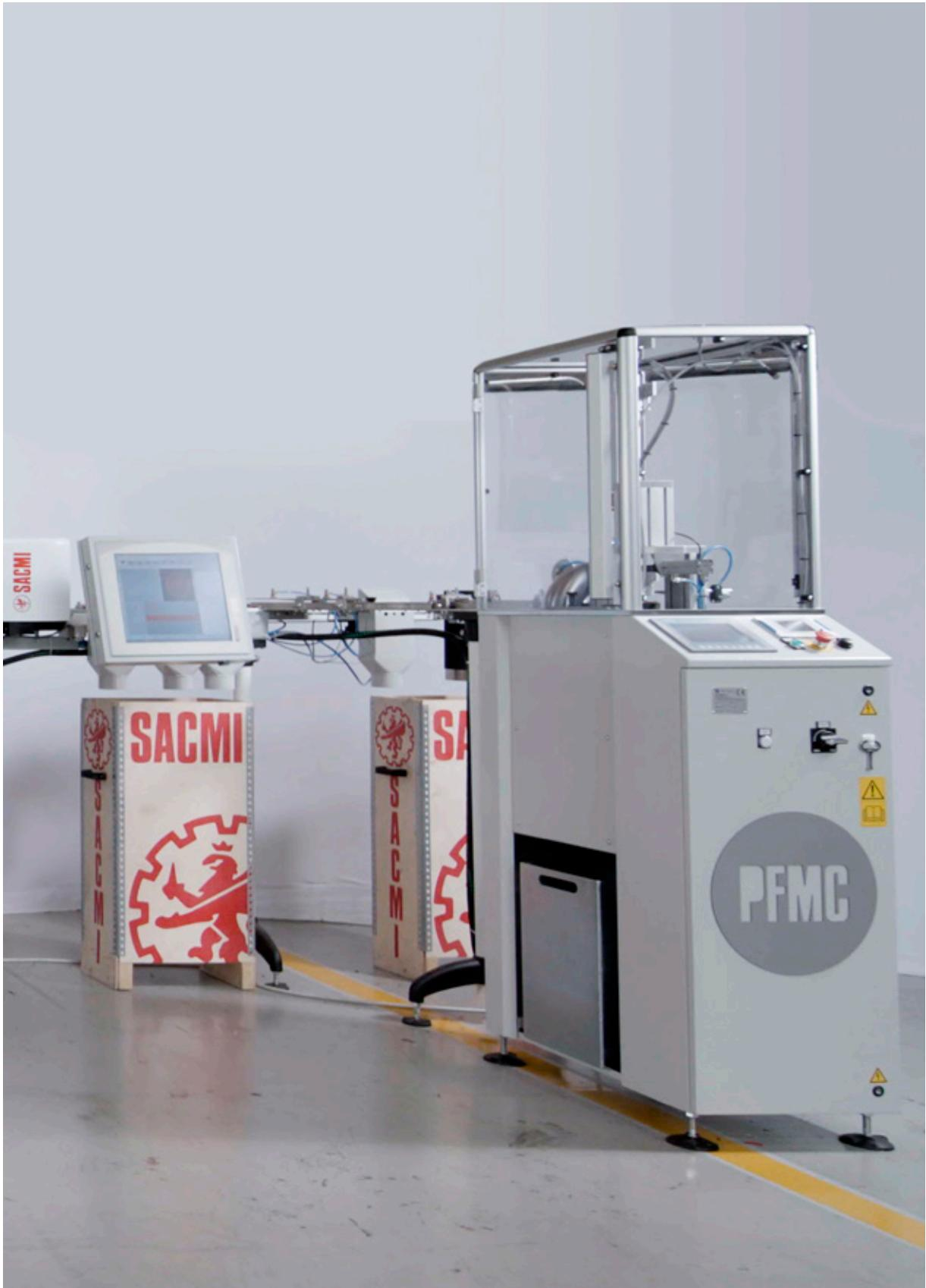
At set intervals, the machine takes a sample of caps from the slitting machine outlet chute (usually once per carousel revolution).
