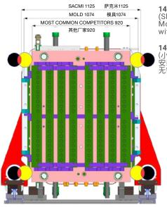
144 cav 45x111 (Short pitch) Mold assembling without rotations
